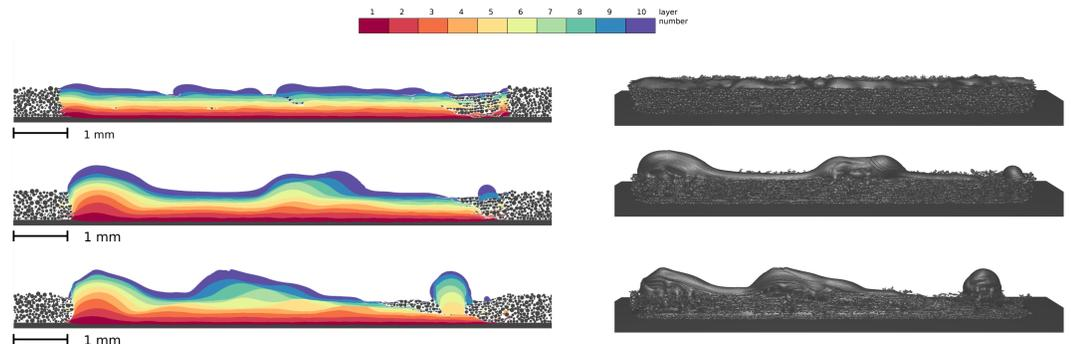
It is shown that the  $\theta_{\text{pow}}$  parameter strongly influences on the wall height and height variation along the wall profile.
