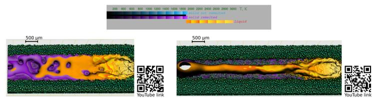
The figure above is a top view of the melt pool during the simulation for the Case 2. If good wetting is set (left figure,  $\theta_{\text{pow}} = 10^\circ$ ), the melt pool widens and shortens. Setting  $\theta_{\text{pow}} = 90^\circ$  leads to the narrowing and elongation of the melt pool.
