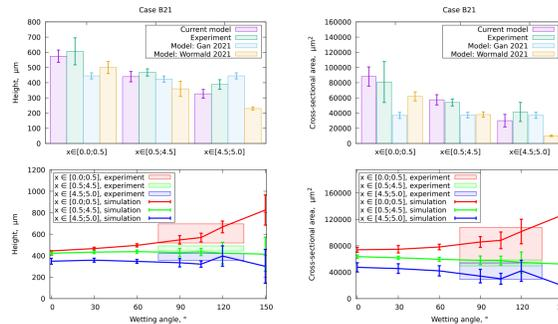
Our model gives very accurate predictions of the thin-wall morphology both in qualitative and quantitative points of view. The thin wall morphology appears to be very strong-dependent on the powder wetting equilibrium angle  $\theta_{\text{pow}}$ . The wall width decreases with the increase of  $\theta_{\text{pow}}$  while the wall height variation and the height in the beginning increases. The paper on this research is submitted in Additive Manufacturing.
