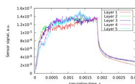
Photodiode sensor signal is simulated during the multilayer simulation. This data could be used for advanced sensor response and feedback algorithms development, including the machine learning algorithms.
