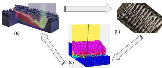
The multilayer EB-PBF simulation takes place as follows. After the layer is simulated in the LBM module (a), the new solidified surface is generated (b). This surface is loaded into the DEM module and used as the substrate for the particles deposition (c). The resulting particle cloud, in turn, used for the simulation for the next layer (a).
